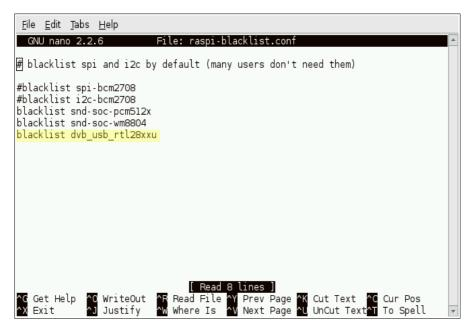
Press <Ctrl>O then <Enter> to save your changes to the file. Press <Ctrl> X <Enter> to exit nano. The line you just added tells the Linux kernel not to load the dvb\_usb\_rtl28xxu device driver when it finds your DVB-T device.
